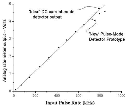
Fig. 4. Prototype detector output at high dose rate.
