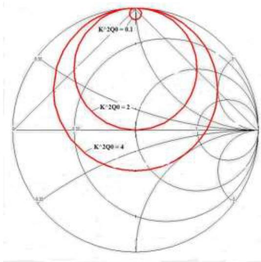
Fig. 4. Q Circles for Various Coupling Parameters
