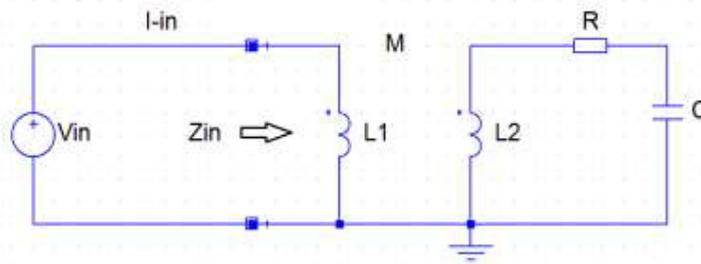
Fig. 1 Equivalent lumped circuit.
